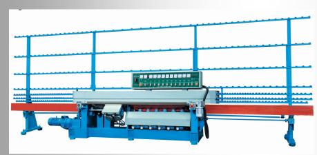
The M&W Ultra Series SAE10M is a 10 spindle variable angle mitering machine, with 2 diamond, 2 resin and 2 polishing spindles on a 0-45° mitering base and 4 spindles for the front and rear arris. The glass thickness is adjusted by turning a knob on the control panel and displayed on a scale meter. The mitering angle is adjusted by turning a knob on the control panel and the
